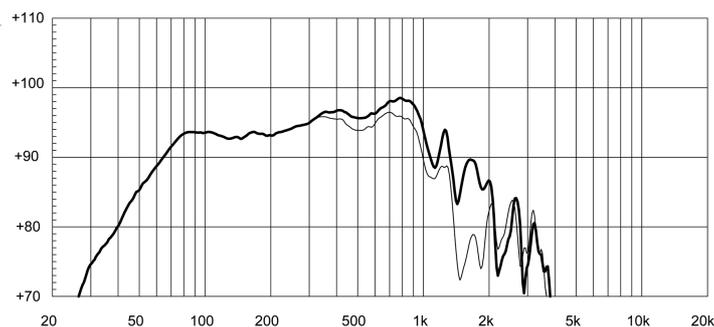
**FREQUENCY RESPONSE CURVE OF 15NLW9500 MADE ON 180 LIT. ENCLOSURE TUNED AT 35HZ IN FREE FIELD (4PI) ENVIRONMENT. ENCLOSURE CLOSES THE REAR OF THE DRIVER. THE THIN LINE REPRESENTS 45 DEG. OFF AXIS FREQUENCY RESPONSE.**
